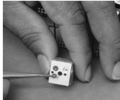
Figure 5.10: DH200 Transducer O-Ring Replacement
